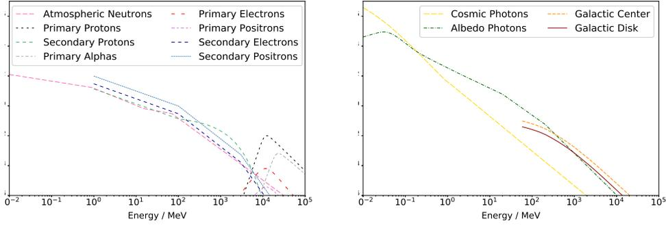
**Fig. 1.** Full on-orbit background spectrum for charged particles and neutrons (*left*) and photons (*right*). All spectra components shown are divided by the solid angle of their region of origin therefore pointing and field-of-view of an hypothetical instrument are not considered.
