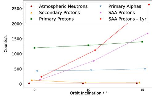
**Fig. 2.** Comparison of the results of the activation caused by the general on-orbit background and by the passage of the SAA, both from the short-lived isotopes, without considering any cool down time, and from the long-live ones. Results are shown for three different orbit inclinations. All the results were calculated for an altitude of 550 km.
